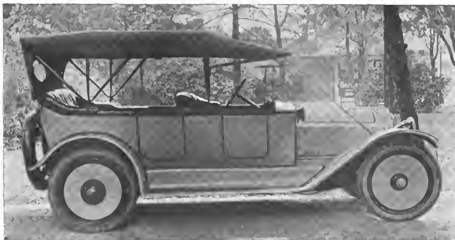
In the experimental car with Putman wheels the disks are painted body color with hubs and rims in darker tint. Note that the tire valves are concealed behind the disks, though this does not hinder their accessibility
